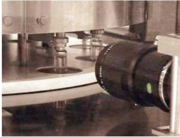
*FIGURE 3. An identification code is print-stamped onto metallic seals after the seals are crimped onto the medicine bottles. Then, the camera acquires the first of two optical-character-verification images of the seals to ensure that they have been correctly marked. This inspection occurs immediately after printing, when the product is paused in front of the camera.*
